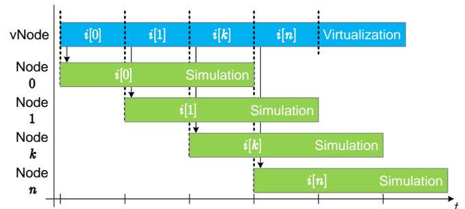
**Figure 1: The workload is executed with virtualization. Checkpoints at the interval boundaries serve as starting points for parallel simulations.**
